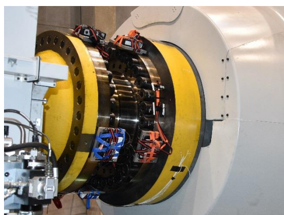
FIGURE 2 TORQUE TRANSFER STANDARD EQUIPPED WITH AN AUTARKIC DATA ACQUISITION.
