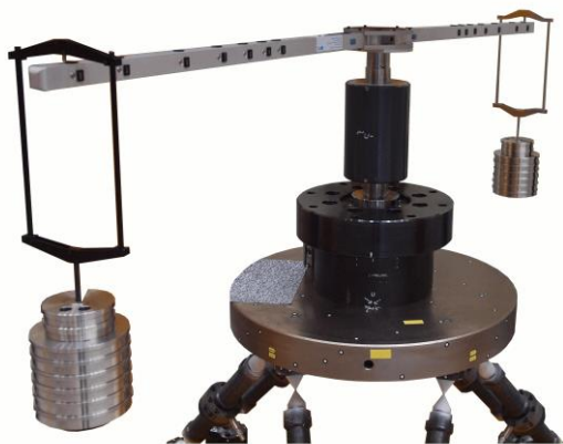
FIGURE 4 LOADING SYSTEM FOR MULTI-COMPONENT INVESTIGATIONS POSITIONED ON PTBS HEXAPOD
