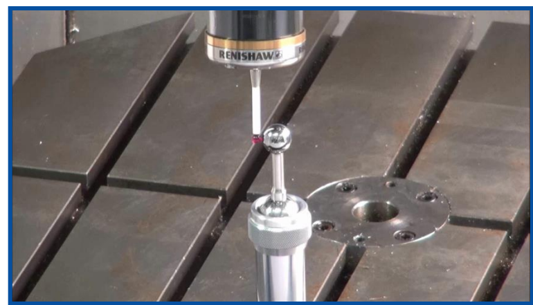
9 probed points in specific approach directions are defined in the MCS
