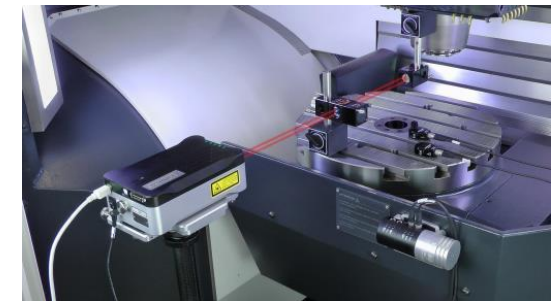
Laser Interferometry (On-line measurement) [Schwenke2005], [Chen1999]
