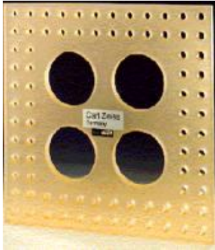
Hole plate [Trapet1991]
