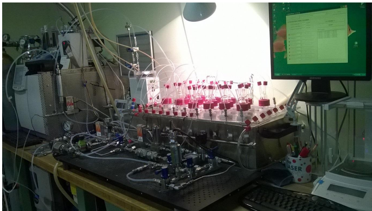
Figure 6: Stationary dynamic generator for trace amount concentrations of AMCs.
