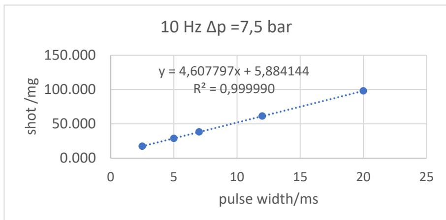
Figure 2.3. Calibration example.
