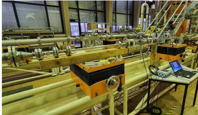
Fig. 2.11: Installation of Coriolis flow meter and needle valve in measuring section.
