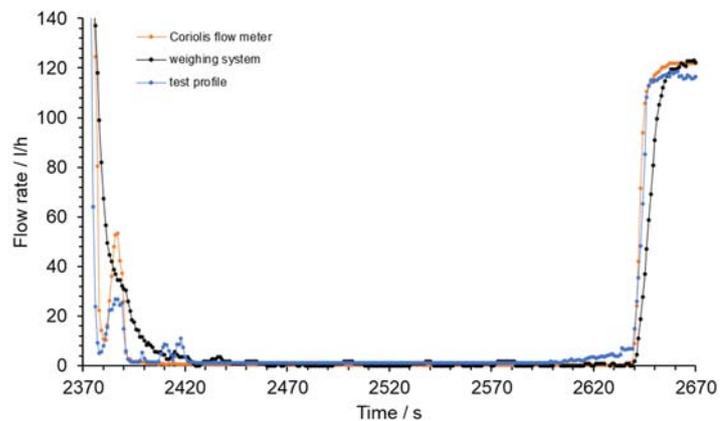
Fig. 3.1: Example of delayed responses of Coriolis flow meter and weighing system with respect to a given decreasing and increasing flow rate change. The data sets were synchronized beforehand.
