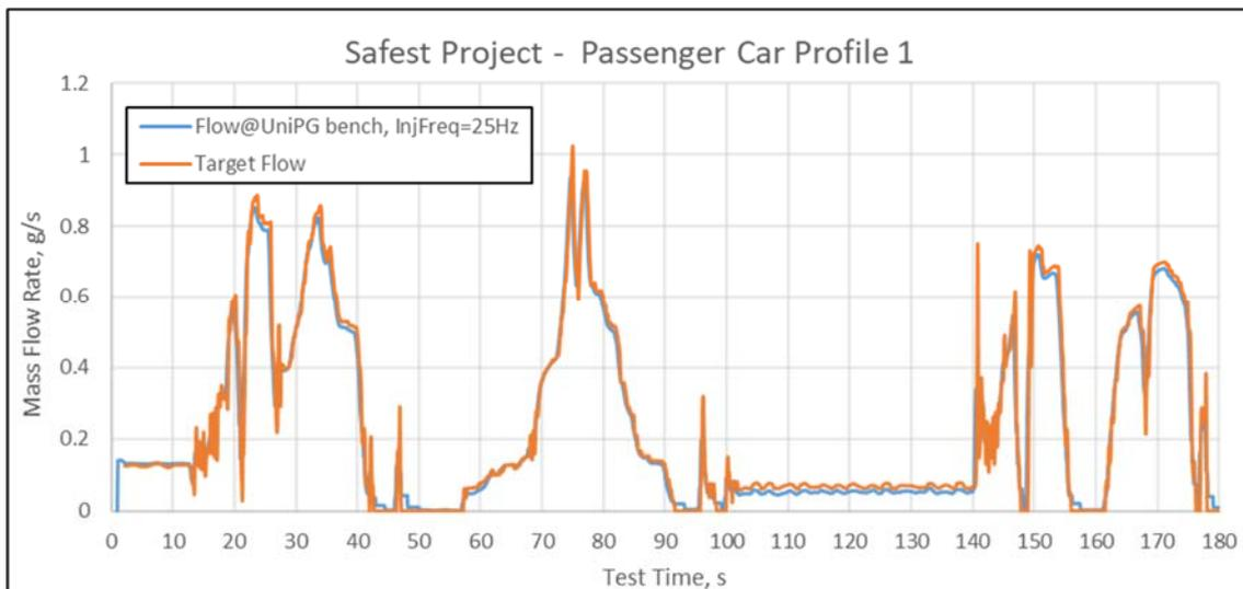
Fig. 2.9: Realization of the Passenger Car Profile 1 with the UniPG test bench
