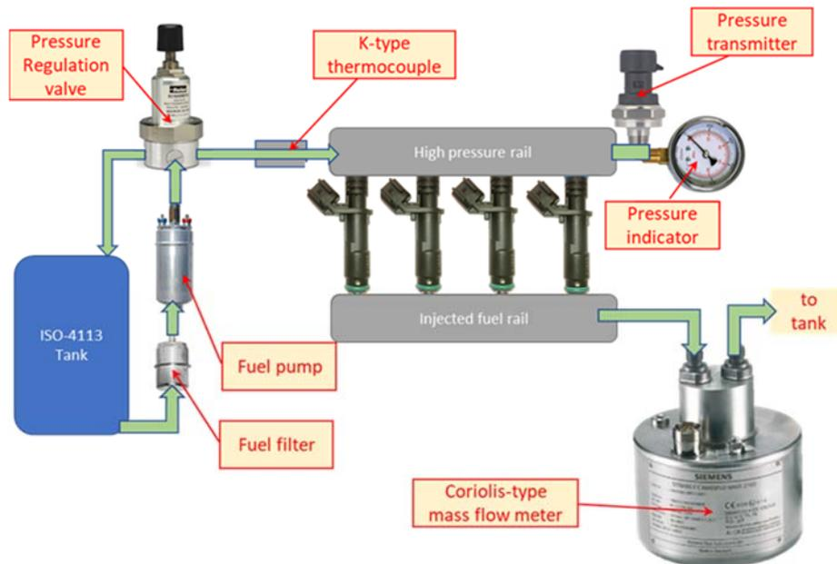
Fig. 2.4: Schematic of the Dynamic Hydraulic Test Bench used.
