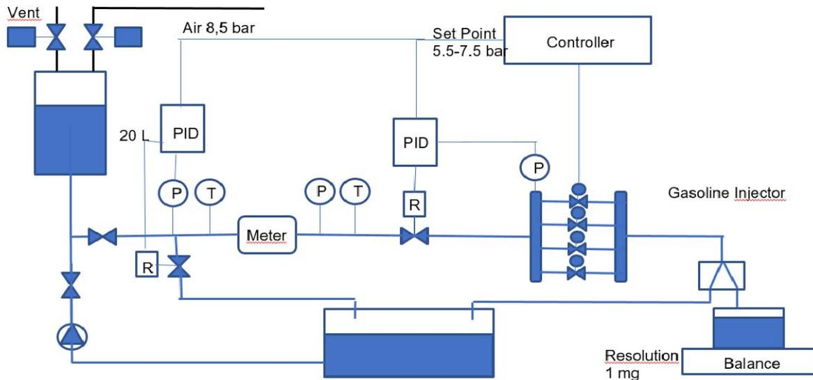
Fig. 2.2: The INRIM test bench for flow meter calibrations
