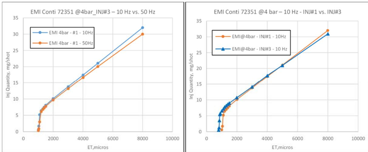
Fig. 2.6: Injector characterization - EMI curves
