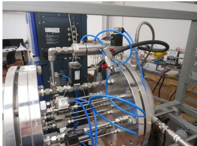
Fig. 2.10: Cavitation nozzle apparatus integrated in a conventional test bench with weighing system as reference.
