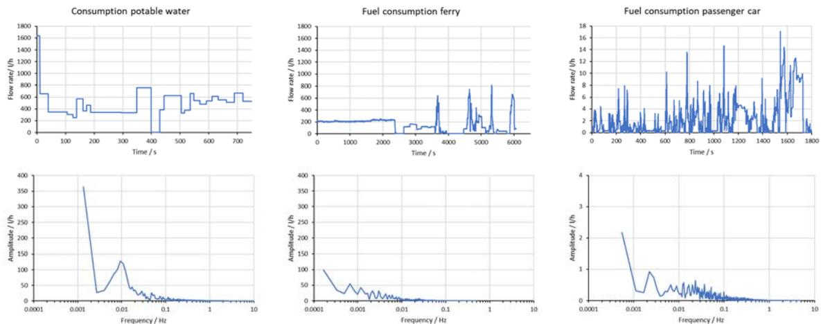
Fig. 2.1: Examples of test profiles for different applications; top: time series, bottom: amplitude spectrum. The profiles are linked to the consumption of potable water in households in Central Europe, to fuel consumption of a ferry navigating in a harbour and the fuel demand of the engine control unit of a passenger car on the basis of the Worldwide Harmonized Light-Duty Vehicles Test Procedure (partially different scaling of y-axes).
