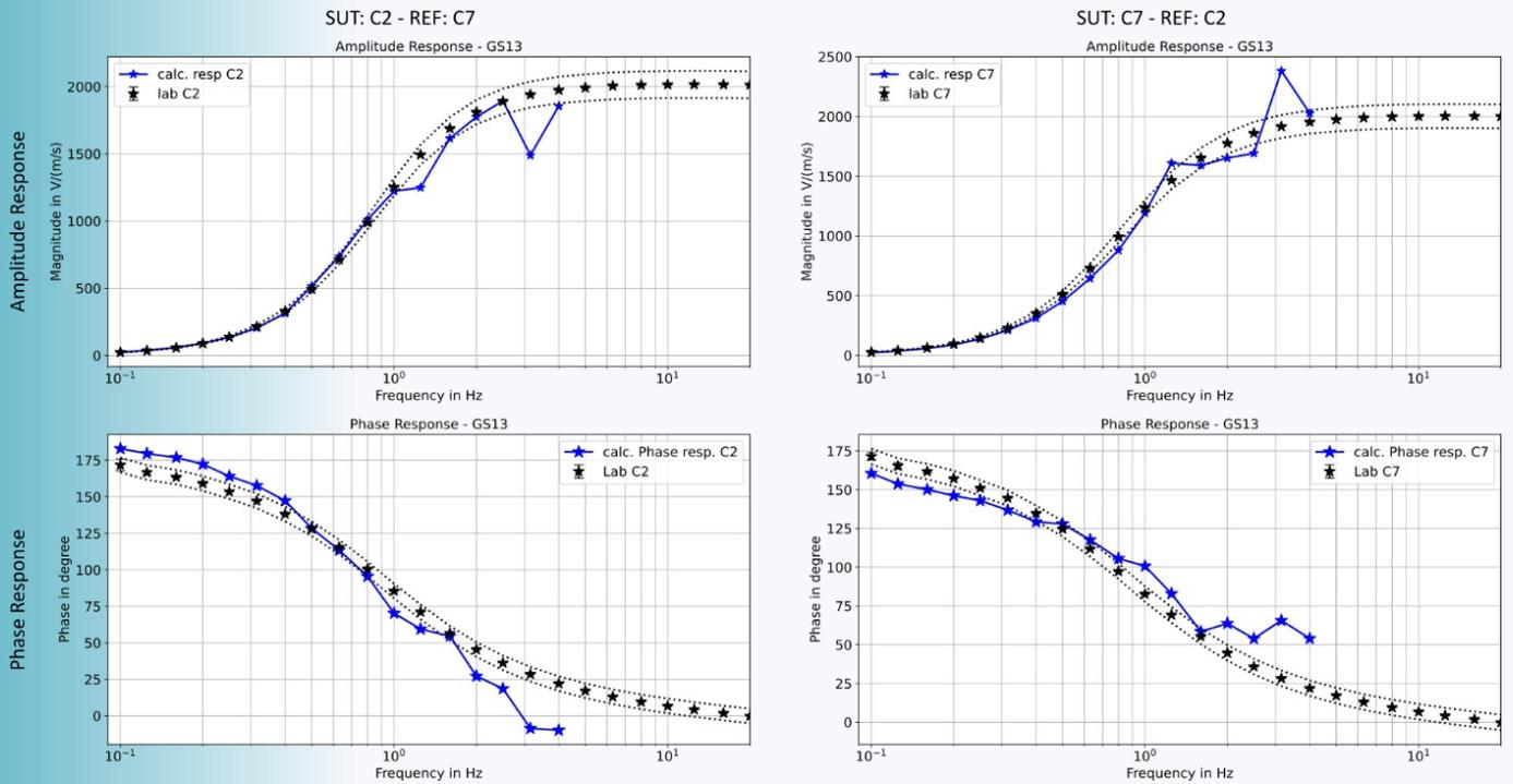
observed for the phase response. Note that when the reference – test sensor pair are exchanged (right column), the phase deviations are mirrored. This indicates an influence of the travel time of the signal between the sensors.
