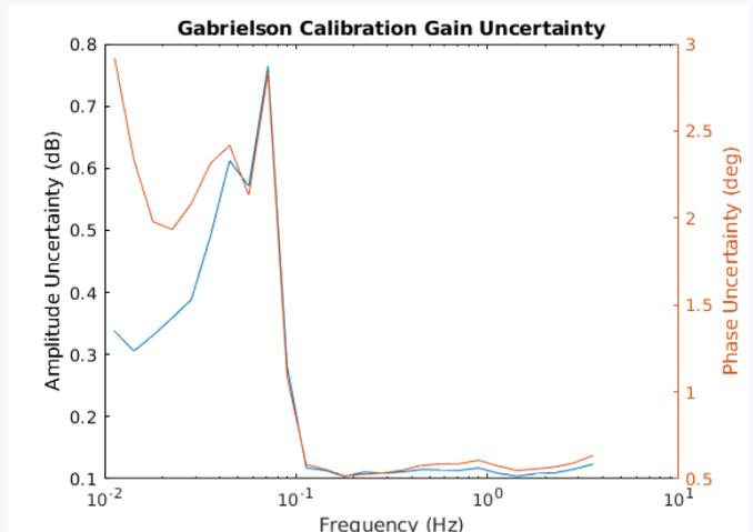
*Gabrielson-Charbit calibration gain uncertainty for the sensor-under-test. The amplitude uncertainties (blue) are provided in dB relative to the total calibration response, and the phase uncertainties (orange) are provided in degrees.*
