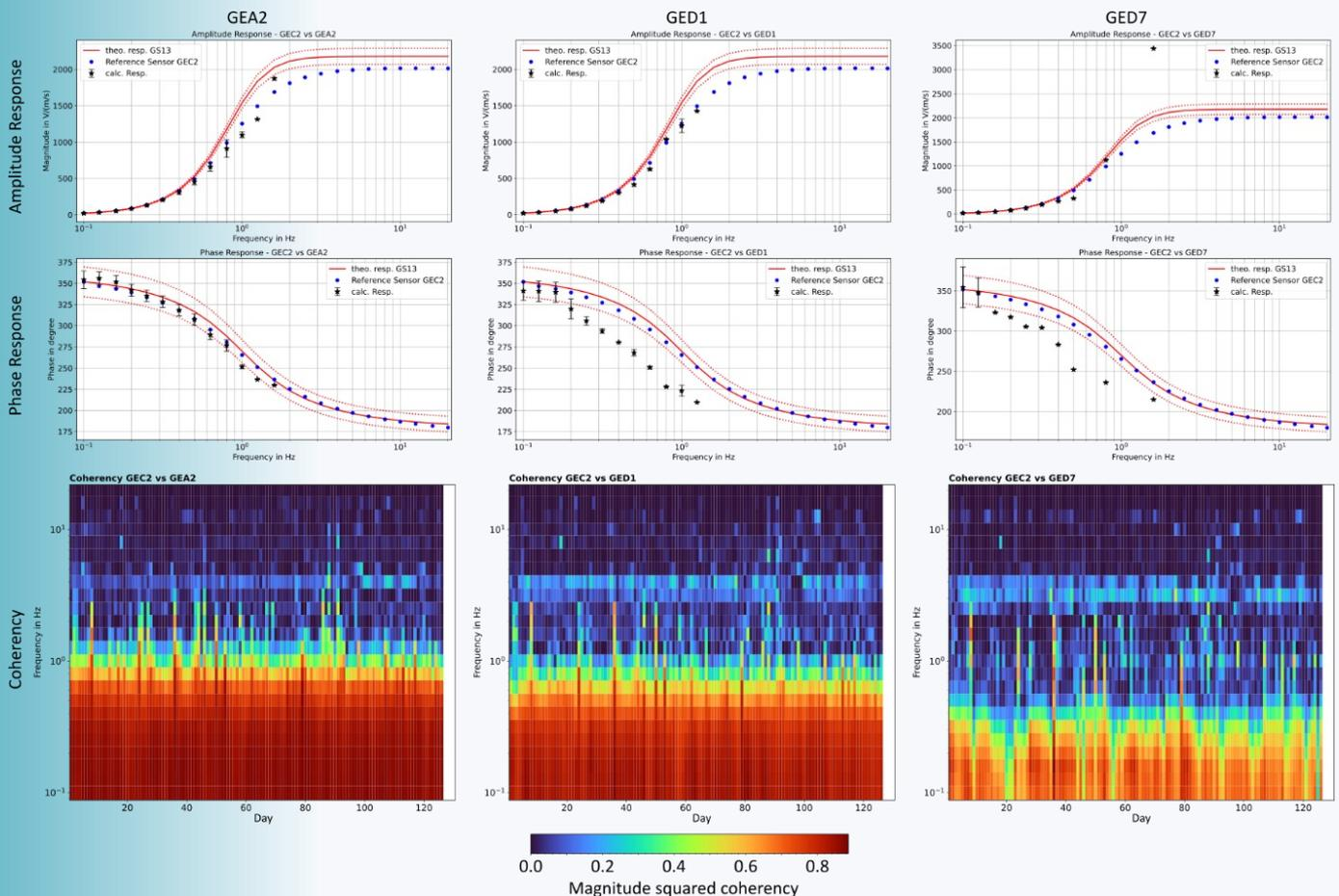
These plots show the results for three sensors (GEA2, GED1, GED7) in varying distances (722m, 1000m, 2900m) to the reference sensor. In the top and middle rows, the amplitude and phase responses are shown (black asterisks), respectively, and compared with the nominal values (red) and the reference sensor (blue dots). The bottom row shows the coherency for each given pair over a 130-day period.
