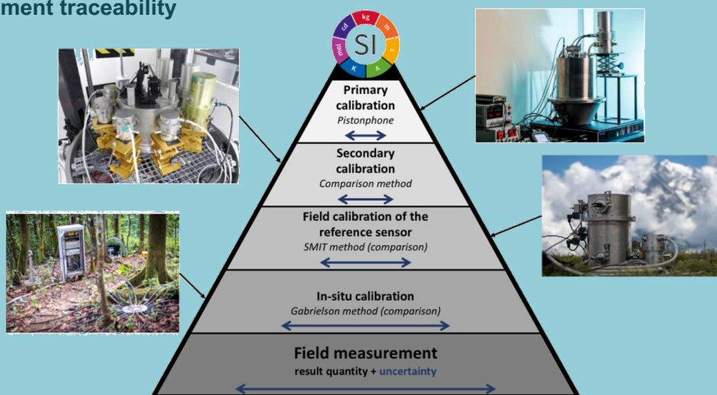
Traceability pyramid linking field measurements to the International System of Units (SI), thus showing how uncertainties in field measurements are inherited from each step, all the way up to the definition of the SI. The arrows represent the order of magnitude of the measurement uncertainties at each step.
