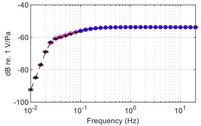
**Left:** Open-circuit pressure sensitivity level (dB re. 1 V/Pa) and uncertainties (dB) of HBK-DPLA (red crosses) and LNE (black stars) for one B&K 4160 microphone. **Right:** Pressure sensitivity level (dB re. 1 V/Pa) and uncertainties (dB) of LNE (black stars) and PTB (blue crosses) for one B&K 4193 microphone
