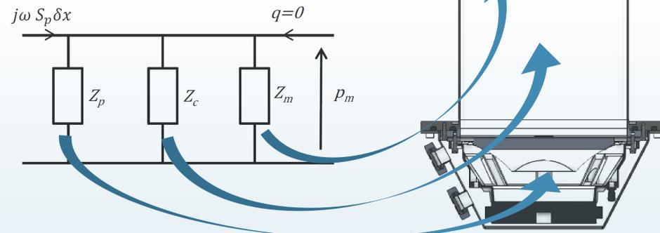
The sound pressure is assumed to be uniform in the coupler (valid for  $\lambda \gg \sqrt[3]{V}$ , i.e. frequencies < 20 Hz).
