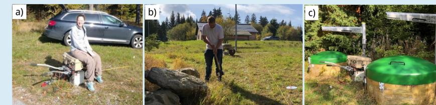
**Fig. 1: Excitation sources in operation. a) portable electrodynamic-vibrator system; b) horizontal hammer blows against rocks; c) EViS between the vaults with the station and reference sensors.**
