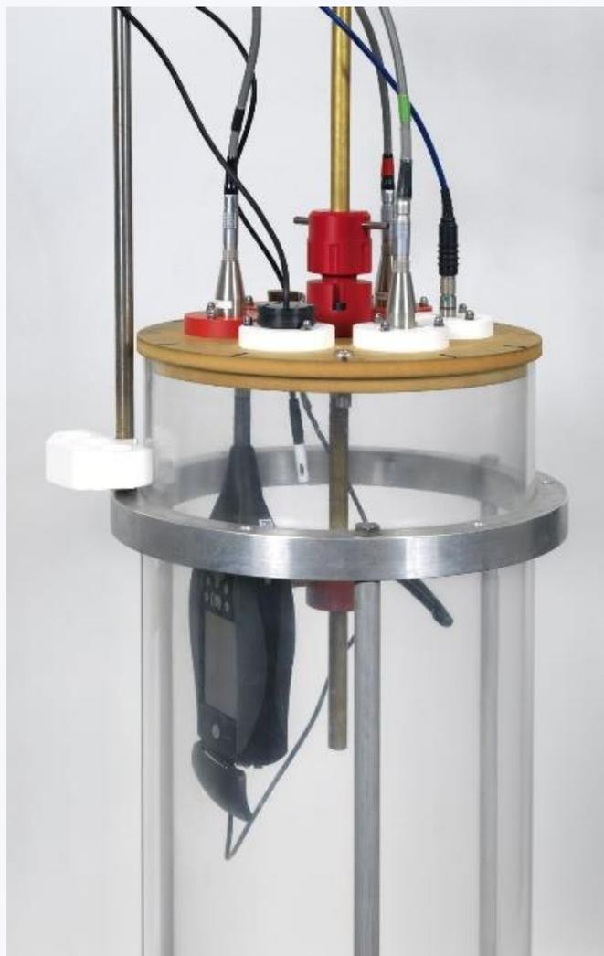
*Acoustical testing of a sound level meter*
