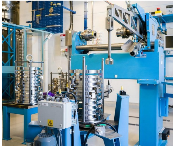
Figure 3: VTT's 2 kN m dead-weight TSM.
