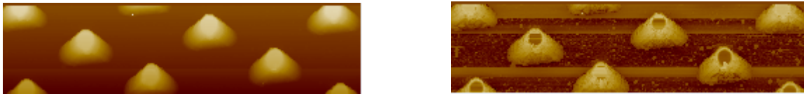
Figure 13: SThM measurement on the TUBS F1-D08-P40 Si nanowires, left: topography, right: thermal signal. Measurements were performed using Park NX-Hivac AFM with resistive SThM module and KNT probe.
