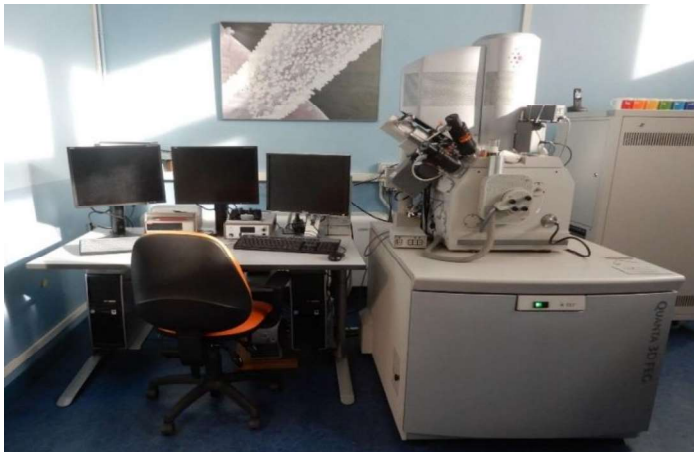
Figure 7. The Dual Beam ESEM FEG Quanta 3D™ used for the NWs manipulation. The microscope is equipped with a Focused Ion Beam (FIB) with a Ga + liquid ion source (gray cylinder inserted at 52° respect to the electron column), two Gas Injector Systems with metallorganic precursors for Pt and SiO x , and four piezo-micromanipulators by Kleindiek Nanotechnik. The beam diameter is 2 nm, it can work with a column acceleration ranging from 1 to 30 kV.
