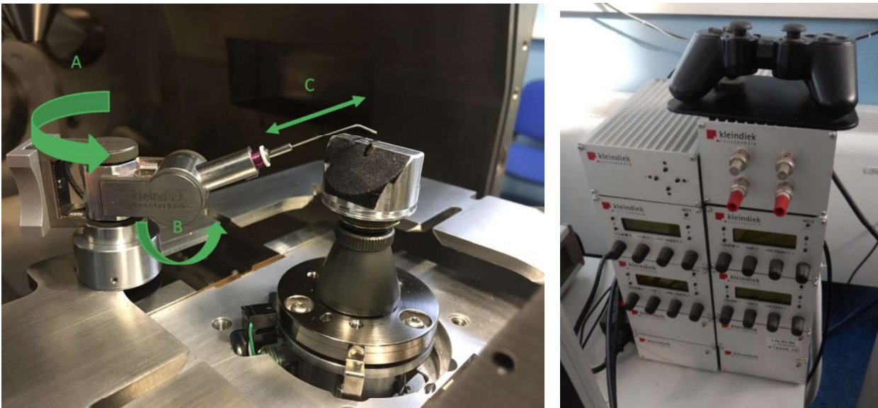
Figure 11. Detail of one of the four Kleindiek MM3A-EM Micromanipulators working inside the Quanta 3D™ chamber (left) and the sample holder. The controllers of the Kleindiek micromanipulators with PS2 pad controller (right). A, B and C are the three movements of the tip: A: horizontal rotation, B vertical rotation, C approaching in the tip direction.
