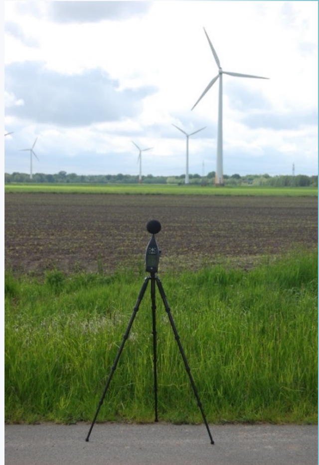
Low frequency noise test measurement at wind park
