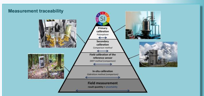
Traceability pyramid linking field measurements to the International System of Units (SI), thus showing how uncertainties in field measurements in inherited from each step, all the way up to the definition of the SI. The arrows represent the order of magnitude of the measurement uncertainties at each step.
