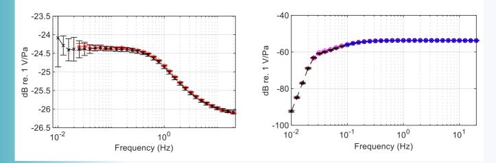
**Left**: Open-circuit pressure sensitivity level (dB re. 1 V/Pa) and uncertainties (dB) of HBK-DPLA (red crosses) and LNE (black stars) for one B&K 4160 microphone. **Right**: Pressure sensitivity level (dB re. 1 V/Pa) and uncertainties (dB) of LNE (black stars) and PTB (blue crosses) for one B&K 4193 microphone
