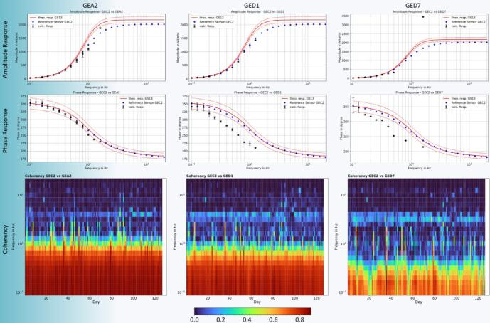
0 0.2 0.4 0.6 0. Magnitude squared coherency These plots show the results for three sensors (GEA2, GED1, GED7) in varying distances (722m, 1000m, 2900m) to the reference sensor. In the top and middle rows, the amplitude and phase responses are shown (black asterisks), respectively, and compared with the nominal values (red) and the reference sensor (blue dots). The bottom row shows the coherency for each given pair over a 130-day period.
