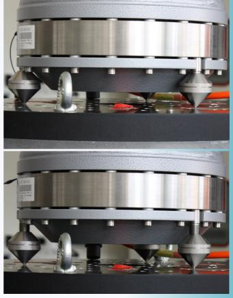
Mounting feet in 'factory' configuration (above) and fully extended (below).
