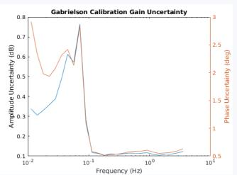
Gabrielson-Charbit calibration gain uncertainty for the sensor-under-test. The amplitude uncertainties (blue) are provided in dB relative to the total calibration response, and the phase uncertainties (orange) are provided in degrees.
