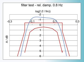
Third-octave band filter at 0.8 Hz plotted as relative damping over normalized frequency on a logarithmic scale and zoomed to the passband area. The filter response measured (in blue) exceeds the acceptance limits (in red).
