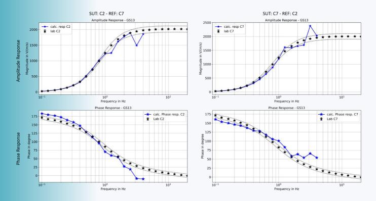
observed for the phase response. Note that when the reference – test sensor pair are exchanged (right column), the phase deviations are mirrored. This indicates an influence of the travel time of the signal between the sensors.
