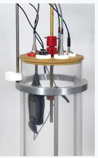
Acoustical testing of a sound level meter
