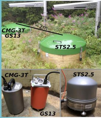
Seismometer installation at PS19
