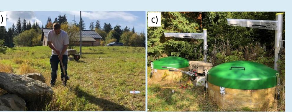
Fig. 1: Excitation sources in operation. a) portable elctrodynamic-vibrator system; b) horizontal hammer blows against rocks; c) ElViS between the
