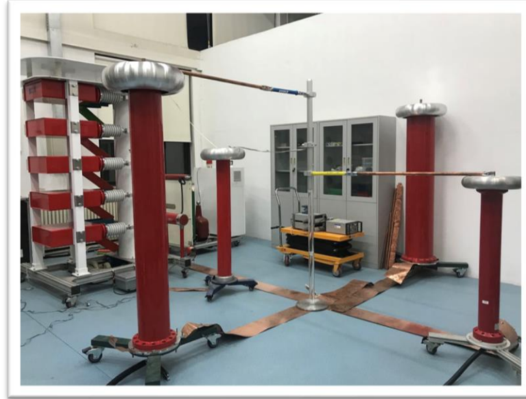
Lightning Impulse voltage
