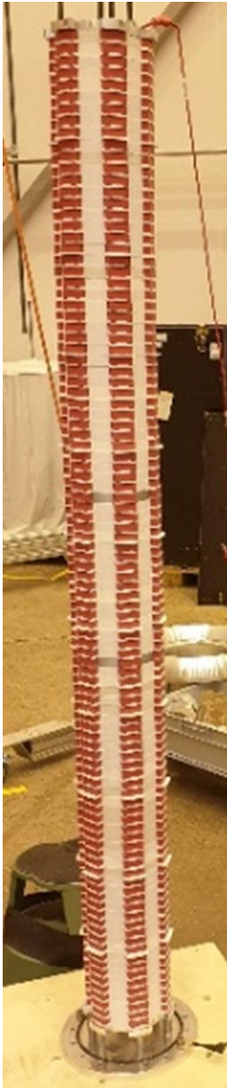
Full 500 kV 100 disc stack
