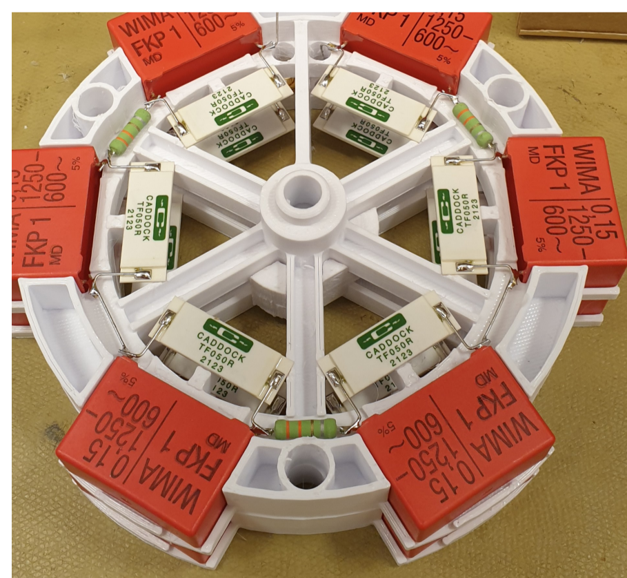
Divider HV construction
