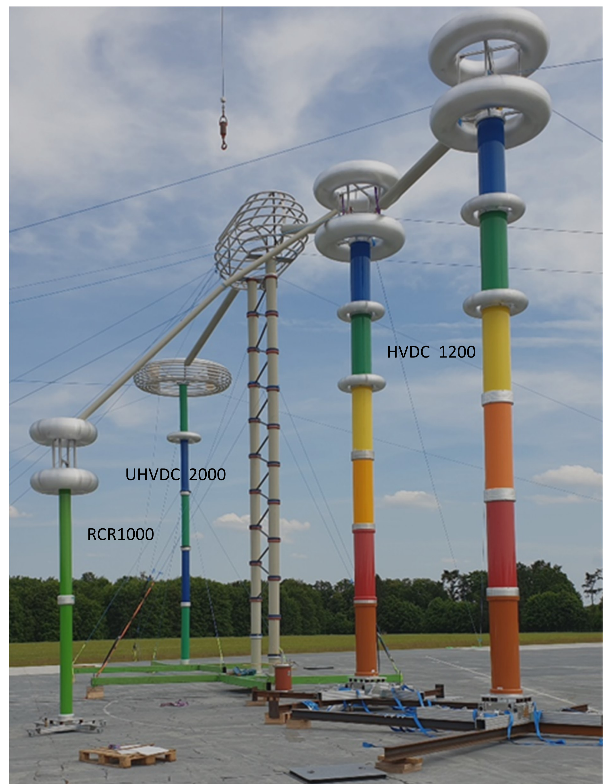
Intercomparison at PTB in June 2022. The universal divider stacked to 1000 kV to the right, two modular HVDC 1200 kV to the left, followed by a new 2000 kV DC generator and the modular UHVDC 2000 kV divider.
