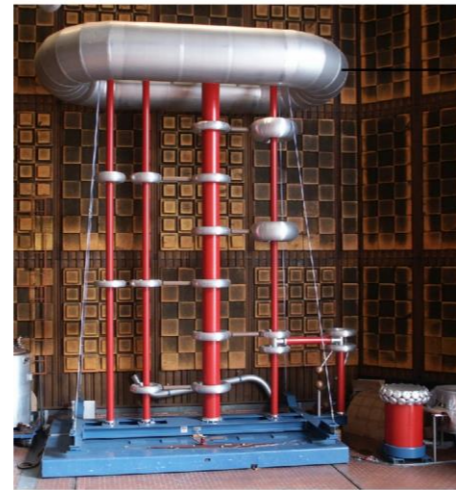
DC: 1500 kV, 20 mA
