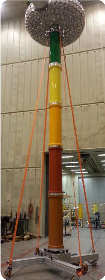
RISE 1000 kV divider at Aalto Finland 2013
