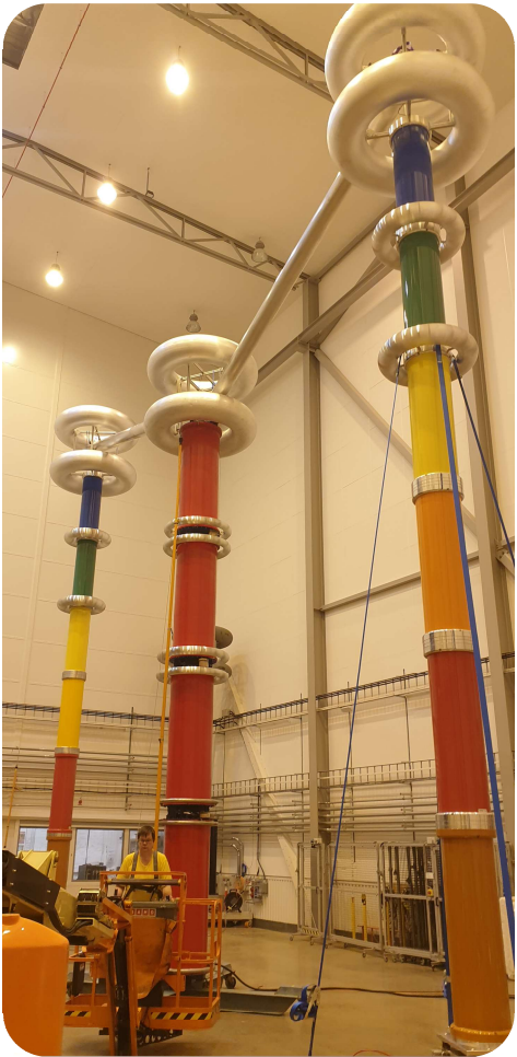
RISE and PTB 1200 kV dividers at RISE 2022
