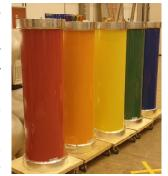
open field at PTB. A complete low ripple 2000 kV UHVDC generator was designed and built by PTB for this purpose. Using the results from the first test has fed into the design and building of a fifth 400 kV module. Characterisation of the compete divider is ongoing for the final campaign with traceable measurement system to 1600 kV,
