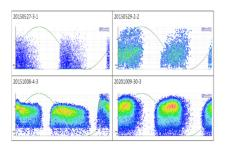
c) PD clustering. These tools allow the determination of the capabilities of PD analysers. These tools must be extended with DC PD patterns.
