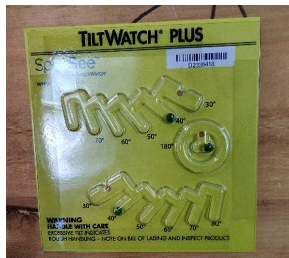
Figure 3. Indicator showing that the EUR-pallet containing the TOP was tilted 40° during transportation.
