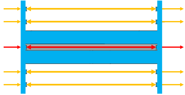
Figure 9. Sketch of the top view of the multi-cavity, as it is prepared at PTB. All parts are made from the same single crystalline type of sapphire with the same crystal orientation. White parts present the evacuated surroundings (outside) and the grey parts present the inner measurement chamber. This multi-cavity therefore has one closed measurement cavity (red beam) and four open reference cavities (orange beams).
