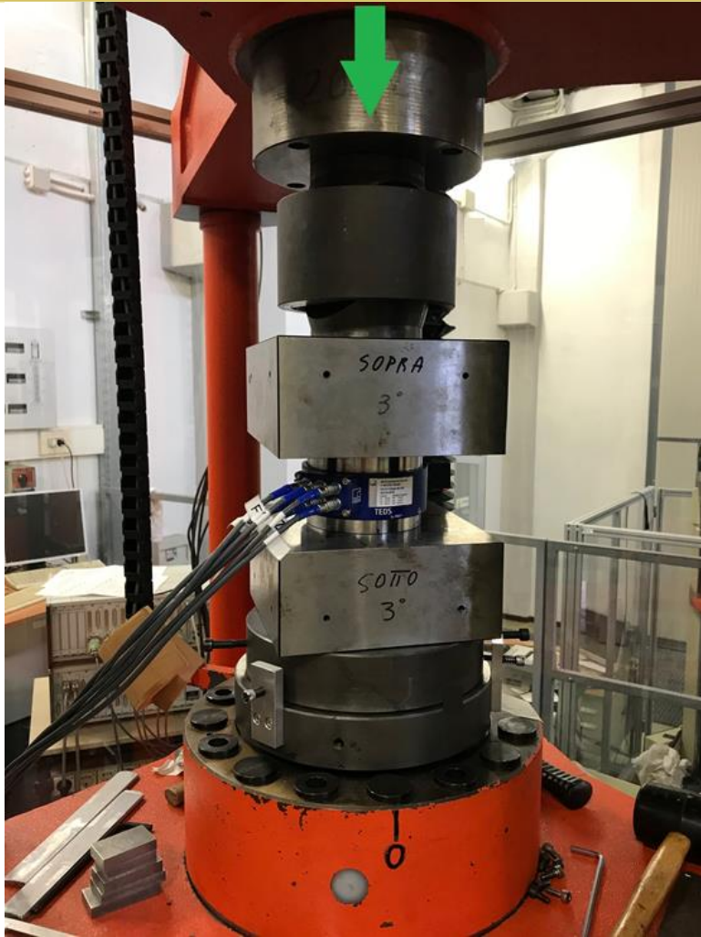
A multicomponent force and moment transducer (MCFMT) during calibration
