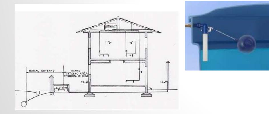
Indirect supply allow the reduction of pessre in the pipes, reducing loss (leakages) and misuse of water (cleaning floor using water jet)
