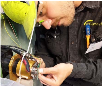
Figure 2. RollResearch scientist installing a microprobe in a roll measuring machine.
