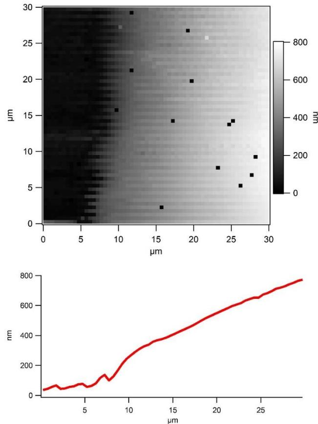
**Fig. 4.** Thickness map and horizontal line profile at  $Y=15 \mu\text{m}$  of a Lupranol film, measured with a sensor shortened to 3 mm length.
