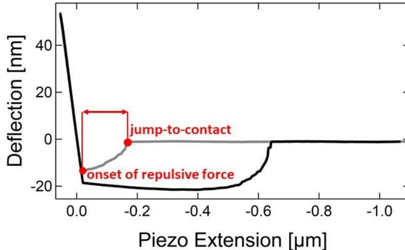
**Fig. 1.** Exemplary force-distance curve on the polyolester Emkarate highlighting the significant points for the determination of thickness. The approach and retraction curves are displayed in grey and black, respectively.
