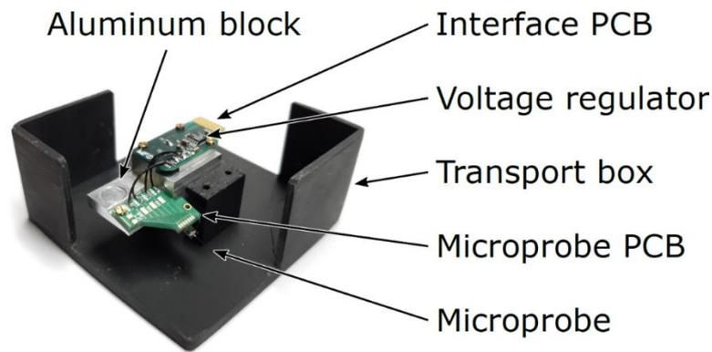
**Fig. 2.** Custom microprobe holder comprising an aluminum body and two PCBs to operate a CAN50-2-5 microprobe in a Cypher S AFM [4].
