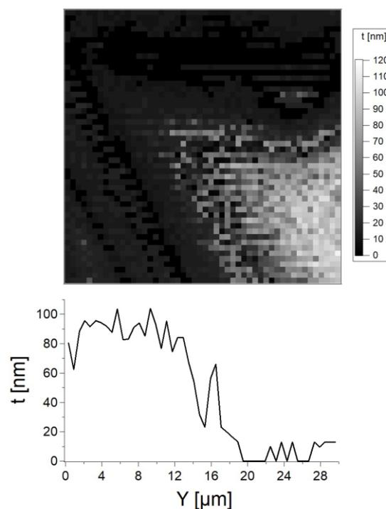
**Fig. 3.** Thickness map and a vertical line profile at  $X=27.8 \mu\text{m}$  of a Lupranol film, measured with a sensor of 5 mm length [4].
