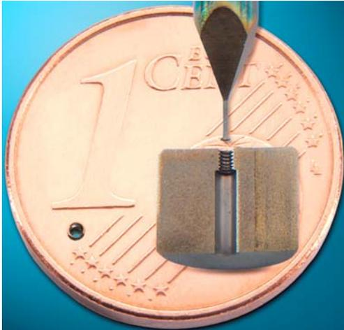
T-shaped microprobe stylus with a probing sphere of 110 µm in diameter, measuring an internal microthread with a size of M 0.7 × 0.175
