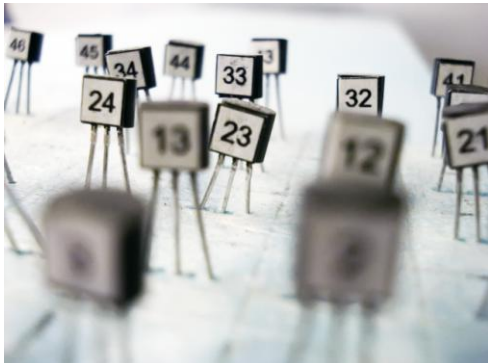
Figure 1: Smallest possible noise thanks to selected field effect transistors
