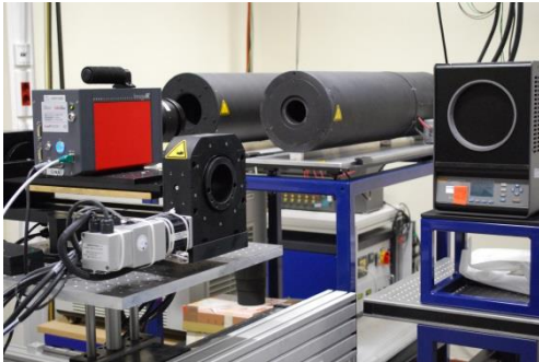
Radiation measuring set-up at PTB for the calibration of thermal radiators and infrared cameras
