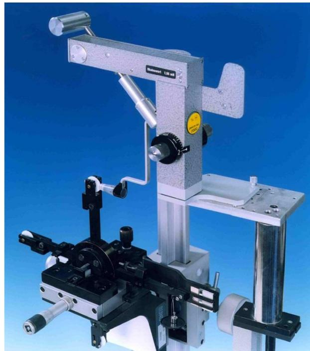
Figure 4.3: Cross beam balance for the verification of applanation tonometers;
