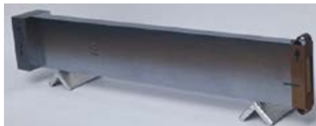
Gauge block made of single-crystal silicon. Dimensions: 197 mm × 35 mm × 9 mm
