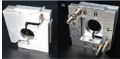
a) Front view of the mirrorholder b) rear view of the mirrorholder
