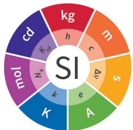
In the new International System of Units (SI), seven fundamental constants will be determined as defining reference entities. The seven base units – arranged in the outer circle of the diagram – will lose their prominent role. (Diagram: BIPM)
