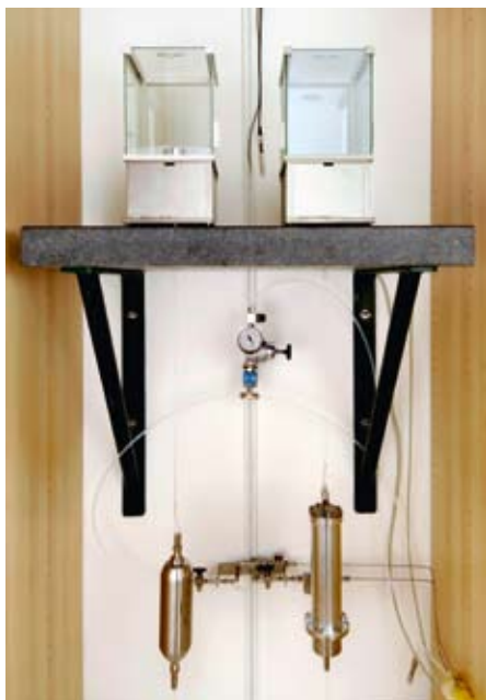
Weighing system to determine the mass flows of ethanol and water
