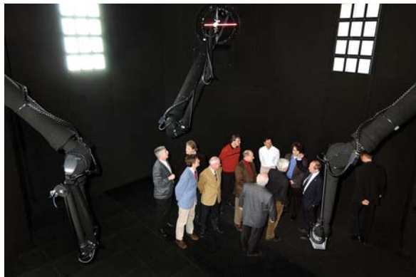
View inside the robot goniophotometer with an LED array as light source in the equipment centre and the two measuring robots in basic position. The group of people provides a size comparison.
