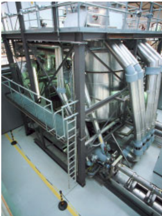
Weighing instrument for gravimetric flowrate determination; max. load: 20 t, measurement uncertainty: 100 g.
