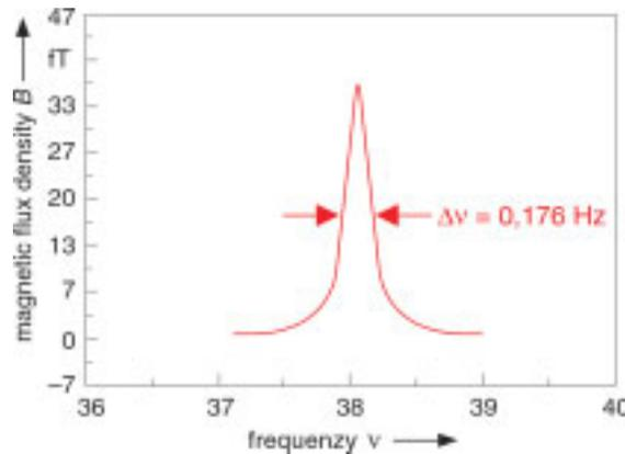
Measured NMR spectrum of distilled water, detection field: 900 nT. Contrary to high detection fields, the natural line width of about 0.15 Hz is broadened only insignificantly by the measuring device.
