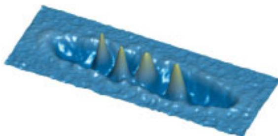
Four Solitons drift in a "channel" defined by light. The soliton diameters are ca. 5  $\mu$ m.
