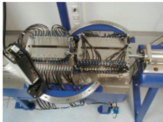
*The new impact-force-standard measuring device. The force transducer is mounted between the two bodies.*
