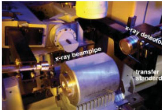
*The new transfer standard with polished mirror (Flat) inside PTB’s Crystal-Orientation Apparatus*
