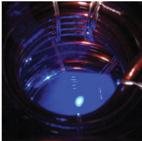
*Fluorescence light from a cloud of Calcium atoms during the first stage of laser cooling.*
