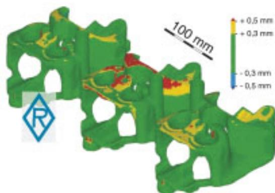
Contour of a water jacket of a cylinder head. The colour-coded surface represents the deviations from the nominal contour in mm. (Source: Fa. Rautenbach, Wernigerode)
