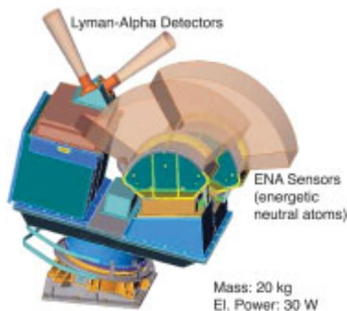
The TWINS instrumentation consists of the Lyman-alpha detectors calibrated by PTB and detectors for energetic neutral atoms.
