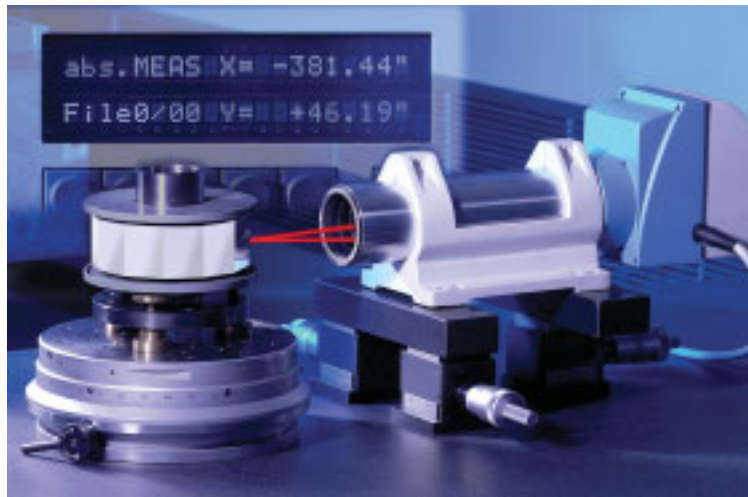
Calibration of a rotary table (index table) with autocollimator and precision polygon
