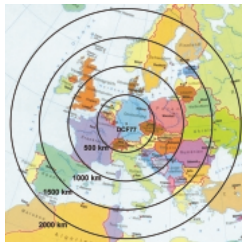
PTB time signals – emitted by the DCF77 long-wave transmitter – can be received by normal radio clocks within a radius of approx. 2000 km.
