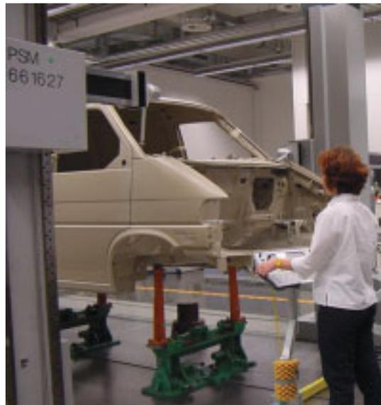
A car body on a large coordinate measuring machine
