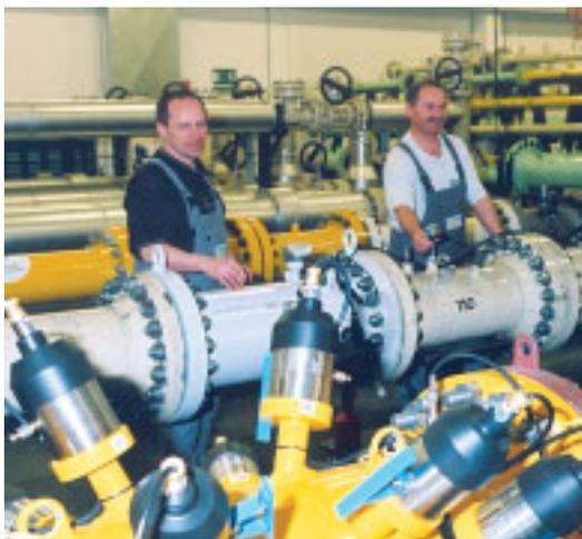
Part of the pigsar team during calibration. The calibrated gas meter can be seen in the front.
