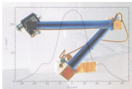
Circular robot for the displacement of a photometer or spectroradiometer in the hemisphere in front of a display for the determination of the values of photometric and colorimetric characteristics and their angular dependence. Plotted is also the luminance as a function of the viewing angle, measured in a horizontal plane in front of a "white-controlled" display (TFT display of a laptop), with strongly decreasing "brightness" at the edge of the viewing area.
