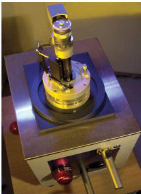
*The  $\beta$ -radiation standard of the PTB for brachytherapy with primary standard measuring device placed on top*
