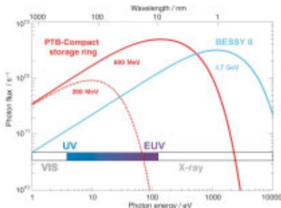
Photon flux of the compact storage ring, compared with BESSY II
