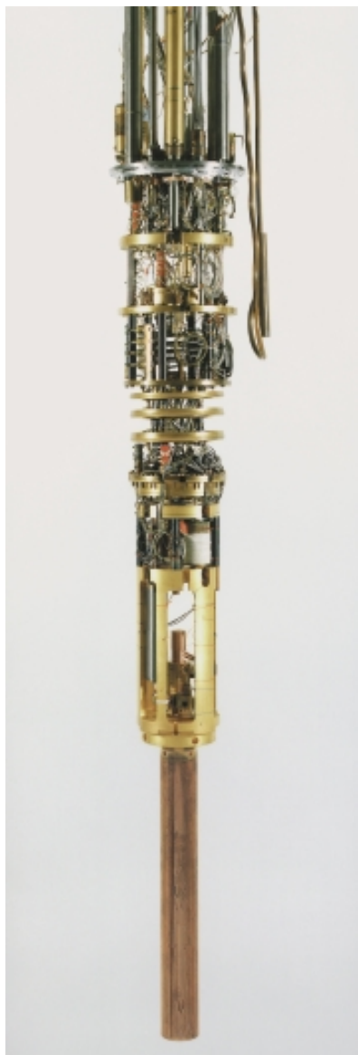
Cryostat insert of PTB used to generate very low temperatures. The nuclear demagnetisation stage at the lower end consists of about 2 kg of high-purity copper. The initial magnetic induction is 8 T. Final temperatures of 65 \mu\text{K} can be generated and long-term temperatures of 300 \mu\text{K} can be maintained.
