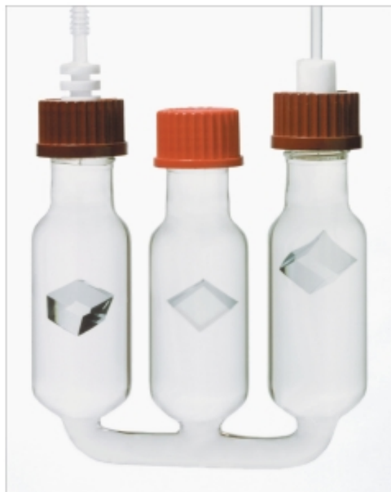
The flotation method allows measuring smallest differences in the density of quartz glass samples. The sample volumes are approximately 1 \text{ cm}^3 .
