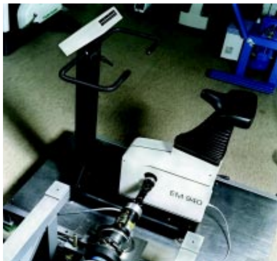
Facility for the measurement of dynamic power at ergometers
