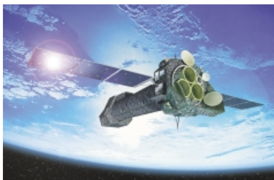
In this artists view of XMM in orbit, the three telescope apertures at the front and the focal-plane instruments box at the end of the observatory are clearly visible. Photo: ESA
