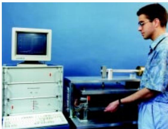
*PTB single sheet tester for the determination of the magnetic properties of electrical sheet steel*
