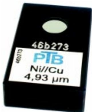
*This coating thickness standard (40 mm × 24 mm × 10 mm) for X-ray measuring devices is made of a 4,93 µm ± 0,1 µm thick nickel coating on a diamond-turned copper substrate. The surface of the coating is exposed and accessible for measurement inside a circle with a diameter of 8 mm.*
