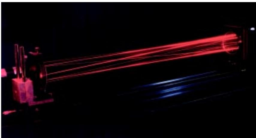
*Multiple path absorption cell for optical partial pressure measurement in the vacuum region, operated in air with a He-Ne laser here*
