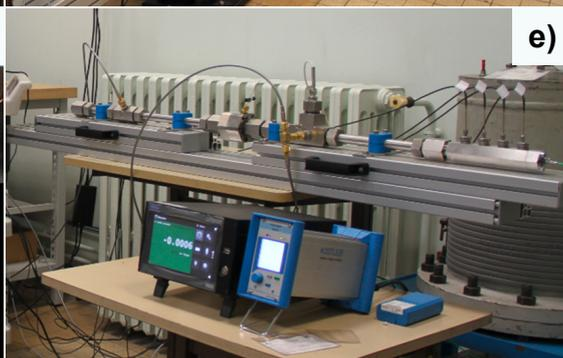
Table 3: Generators of pressure used for the 0.5 MPa range calibration
