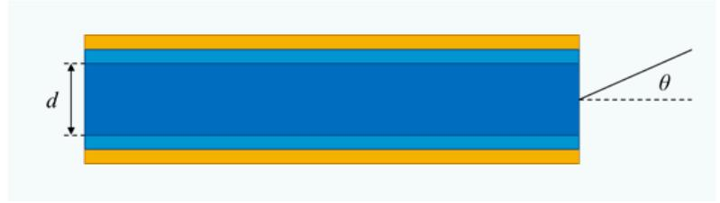
Figure 3: Geometry of the end of the sensor (Au-coated fiber):  $d$  = fiber core diameter;  $\theta$  = maximum acceptance half-angle
