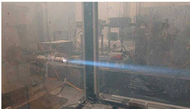
Figure 4: A UV-VIS light beam is transmitted through the soot cloud after a pyrotechnic explosion at NPL. The light is focused into the fiber connected to a spectrometer.
